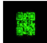
Figure 7 . QR printed on using deer hide up converting nano particle Inks.
