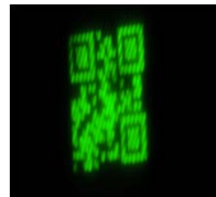
Figure 6 . QR code printed on turkey Feather using up converting nano particle Inks.
