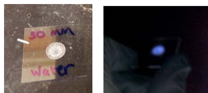
Figure 4: Coverslip spotted with 30 mM tryptophan solution. Taken with cell phone camera under ambient light (left). Taken with modified camera under 305 nm light (right).
