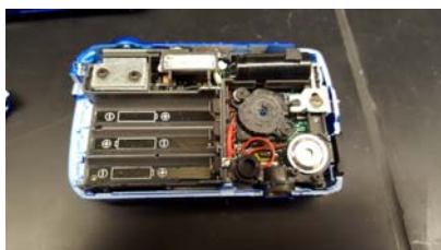
Figure 2: Vivitar Vivicam F126 with UV/IR filter removed in order to capture UV light.
