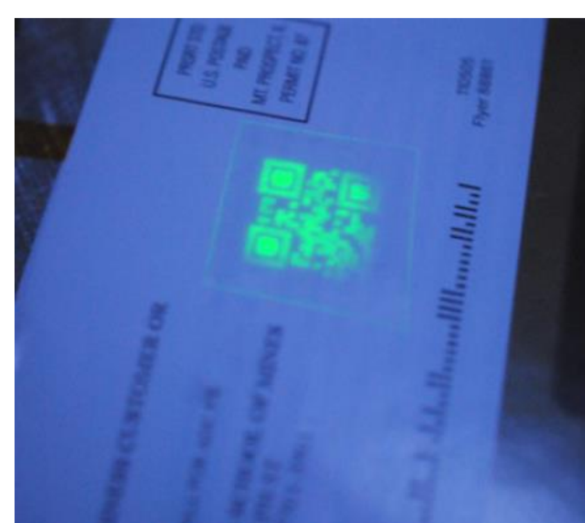
Figure 1: Demonstration of a quick response code printed with upconverting ink using an aerosol jet printer.
