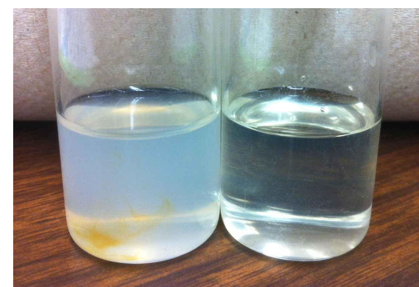
Figure 2: A stable ink on the right compared to an unstable one on the left.
