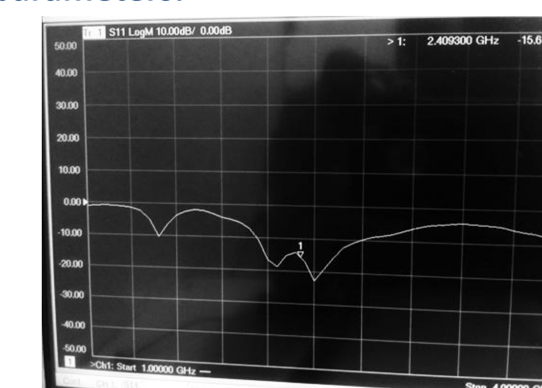
Figure 6: Resonance coefficient of photo-sintered antenna, resonating at 2.4 GHz
